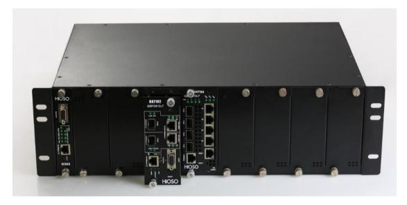
HA7000 is HIOSO EPON rack. HA7000 adopts 19 inch, 3U height rack, supports dual-power supply. The rack supports 8pcs HA7102CS/HA7104 OLT cards, from 2PON to 32PON ports.. Each PON supports 32pcs ONU access within 20KM (maximum 64pcs ONU access within 10KM). It supports integrated management through the network management card M7000.
